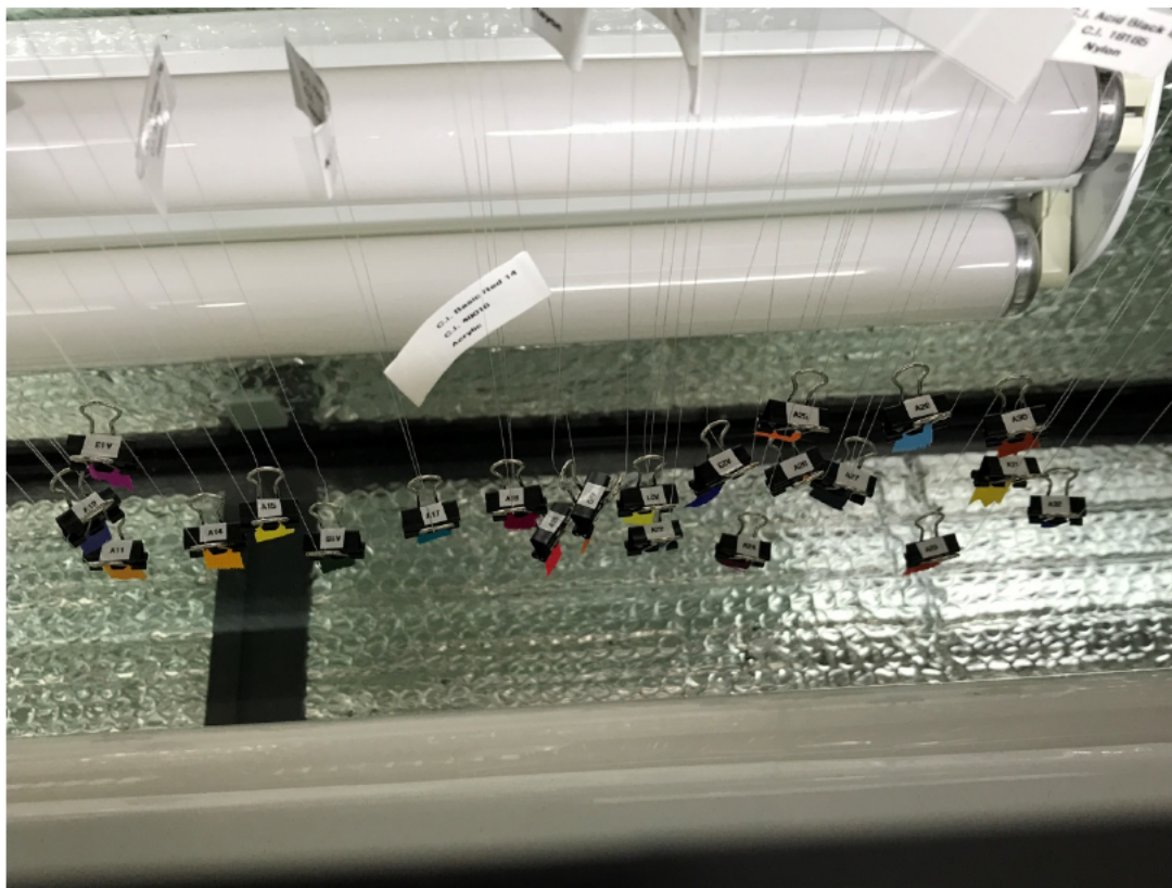
Figure 3. Microtrace fabric swatches inside the UV-radiation light box at McCrone Research Institute, Chicago, October 2017.
