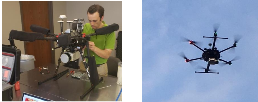
Figure 3. (Left) Installing the A-Series 60 on the M600; (Right) M600 in flight
