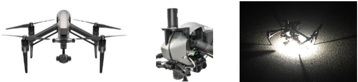
Figure 2. (Left) DJI Inspire 2 with X4S; (Middle) AirGon Loki Direct Geopositioning System; (Right) Inspire 2 at night
