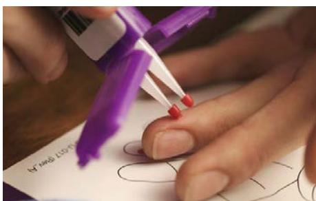
Figure 21: Mitra, offered by Neoteryx, uses a microsampling technology to simplify remote blood specimen collection by collecting blood without a syringe. (Image provided by Neoteryx, LLC)
