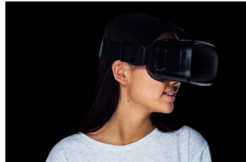
Figure 18: The Tobii VR4 Eye Tracking Platform leverages the HP Reverb G2 Omnicept Edition to enable detection of eye movements and measurements of pupil dilation (pupillometry,) which can be used together with input from a photoplethysmography sensor for measuring heart rate. (Image provided by Tobii)
