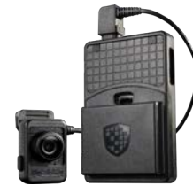
Figure 11: Digital Ally's FirstVU HD body camera uses a two-piece design to reduce the footprint and offer multiple mounting options. The camera head offers 720p HD resolution and a 95-degree angle horizontal field of view, captures HD audio, and is water resistant. (Image provided by Digital Ally)
