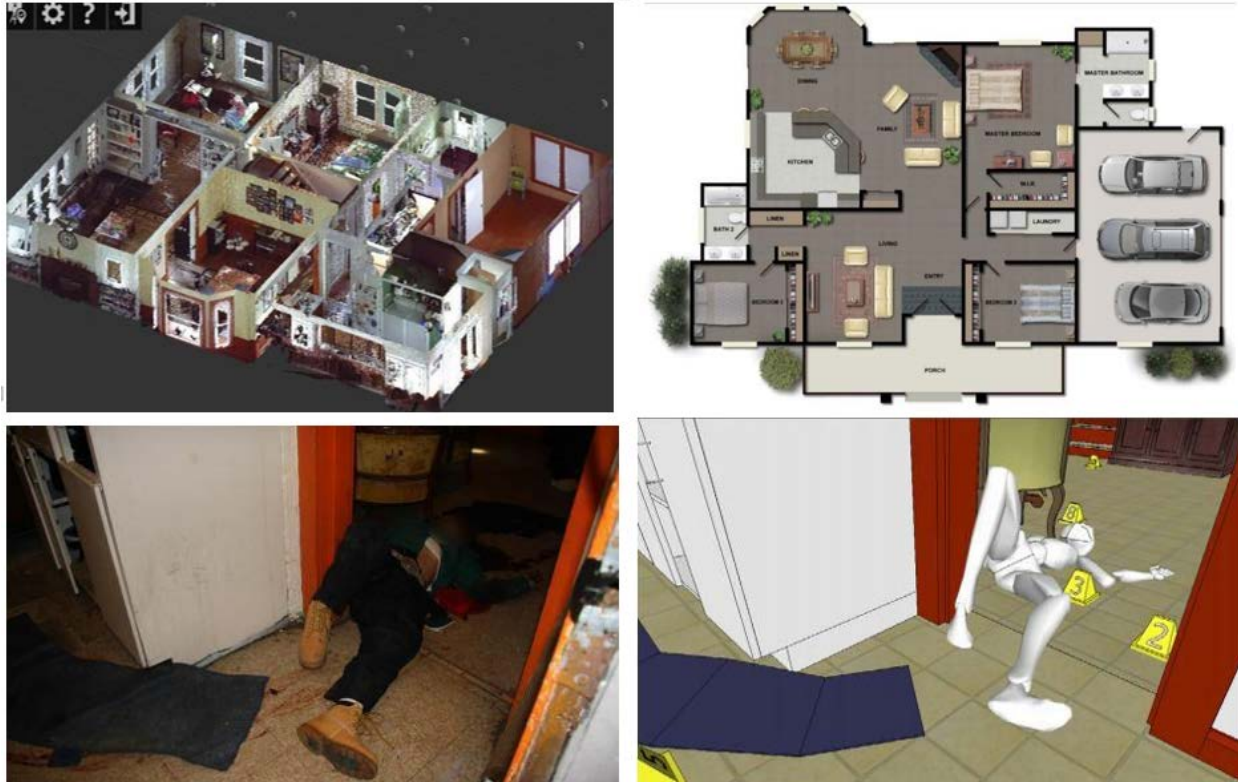
Figure 4: 3D model of a house created using the Faro Focus 3D (Top left) vii , 2D Floorplan created using traditional methods (Top right) viii , Photograph of a body at a crime scene (Bottom left) ix , and a 3D reconstruction corresponding with the previous photograph (Bottom right) x
