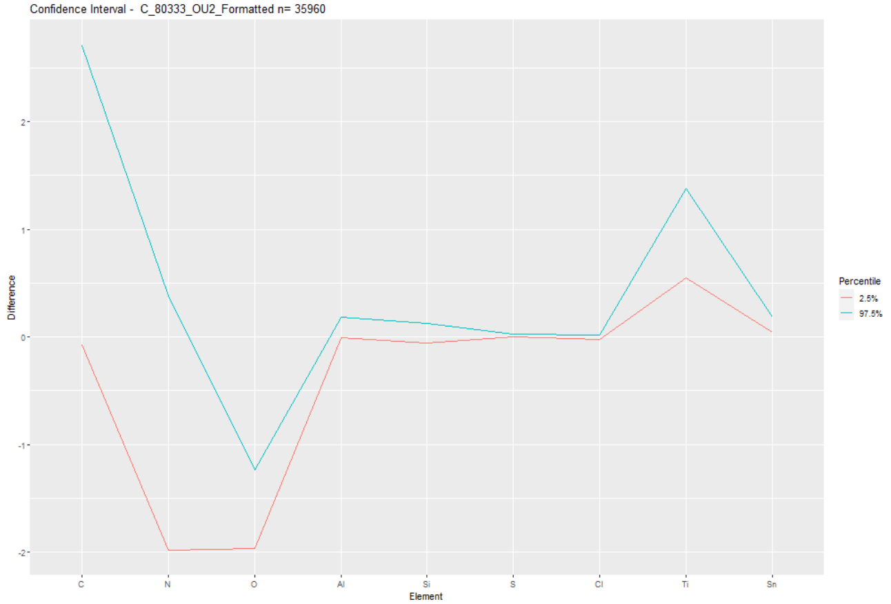
Figure 22. Paint layer 80333 OU2, low degree of heterogeneity. The 95% data window for all 35960 combinations of four 300 \mu\text{m}^2 spectra.
