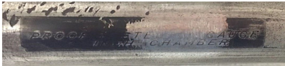
Figure 3.4 Defaced stamped numbers (1 and 2) on a gun barrel [1]
