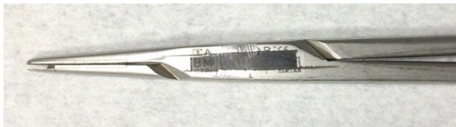
Figure 3.6 Defacing 0,3,4 and R of a laser engraved serial number on a surgical needle handler [1]
