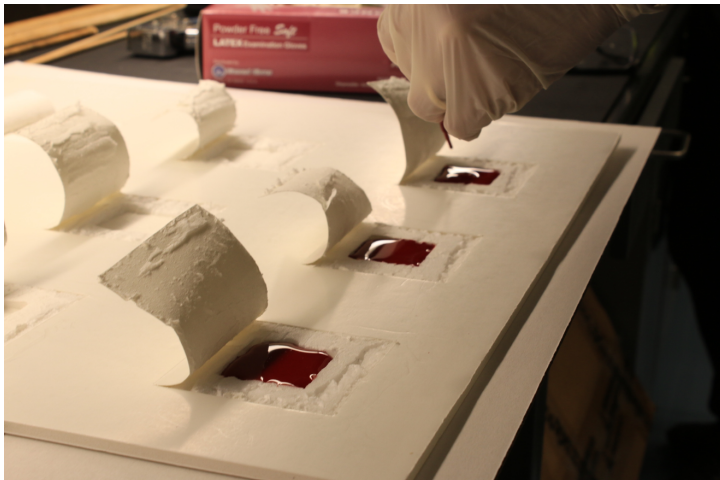
Figure 1. Foam core pockets used as bullet targets
