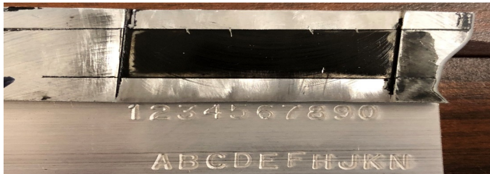
Figure 14. Picture of defaced CTS zinc test sample after sanding and applying black paint.
