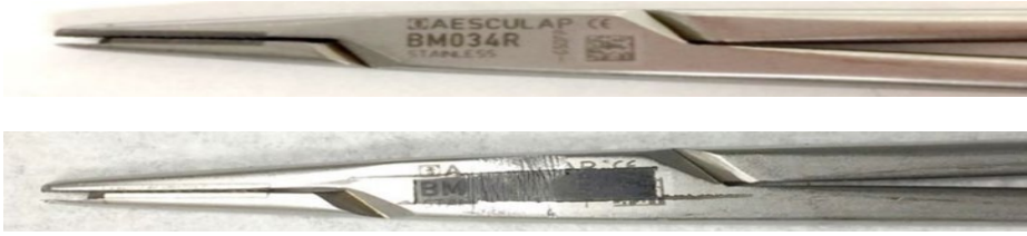
Figure 49. Picture of Forceps before and after the serial number was defaced.
