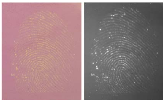
Fig. 18: Fresh, natural fingerprint lifted from glass with a phenol red-impregnated membrane. The membrane had been stored in an airtight container in the presence of sodium polyacrylate beads (previously swelled in water) for one year before use. Visualization was achieved under ambient white light (left) and under 445 nm excitation combined with a 550 nm BBF (right), respectively.
