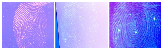
Fig. 4: Marks lifted from glass using membranes functionalized with, from left to right, DFO, indanedione, and fluorescamine. DFO and indanedione were immobilized on positively-charged nylon, fluorescamine on PVDF. Visualization was under UV light.
