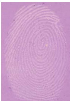
Fig. 17: Three-week-old, charged fingerprint lifted from glass using a phenol red-impregnated membrane lifter that had been stored for two months with a hydrogel cover in a vacuum-sealed pouch. The hydrogel consisted of 5% agarose in 2 mM NaOH containing 0.1% benzalkonium chloride as a preservative.
