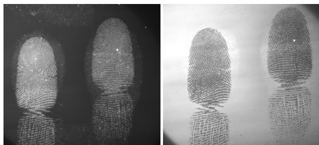
Fig. 5: Directly deposited fingerprints on a phenol red lifter illuminated using (left) an excitation wavelength of 450 nm combined with a 555 nm bandpass barrier filter (BBF) and (right) excitation at 555 nm and observed with a 610 nm BBF.
