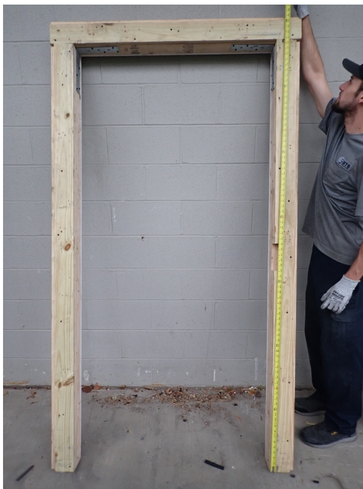
Figure 2 – Simulated Wall Structure for Door Installation
