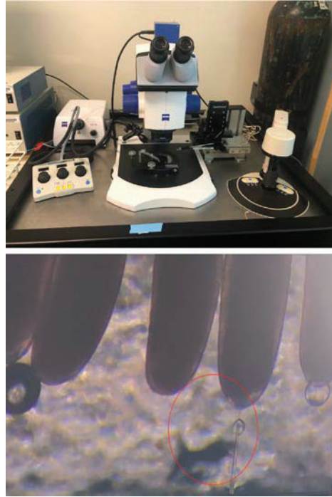
Figure 1. P. regina embryos were injected at the posterior end (see second egg from right) with a Zeiss SteREO Discovery.V8 (Zeiss, Jena, Germany) paired with a Sutter Instrument® Xenoworks micromanipulator and digital microinjector model (Sutter, Novato, CA) and using a borosilicate needle.
