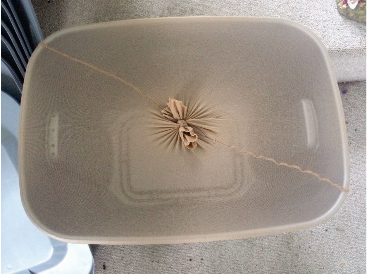
Figure 8. A plastic garbage bin sealed with a sleeve made from pantyhose. We found that reared in an animal carcass placed on a layer of wood shavings in the bin could not penetrate the sleeve after crawling up the side of the bin.
